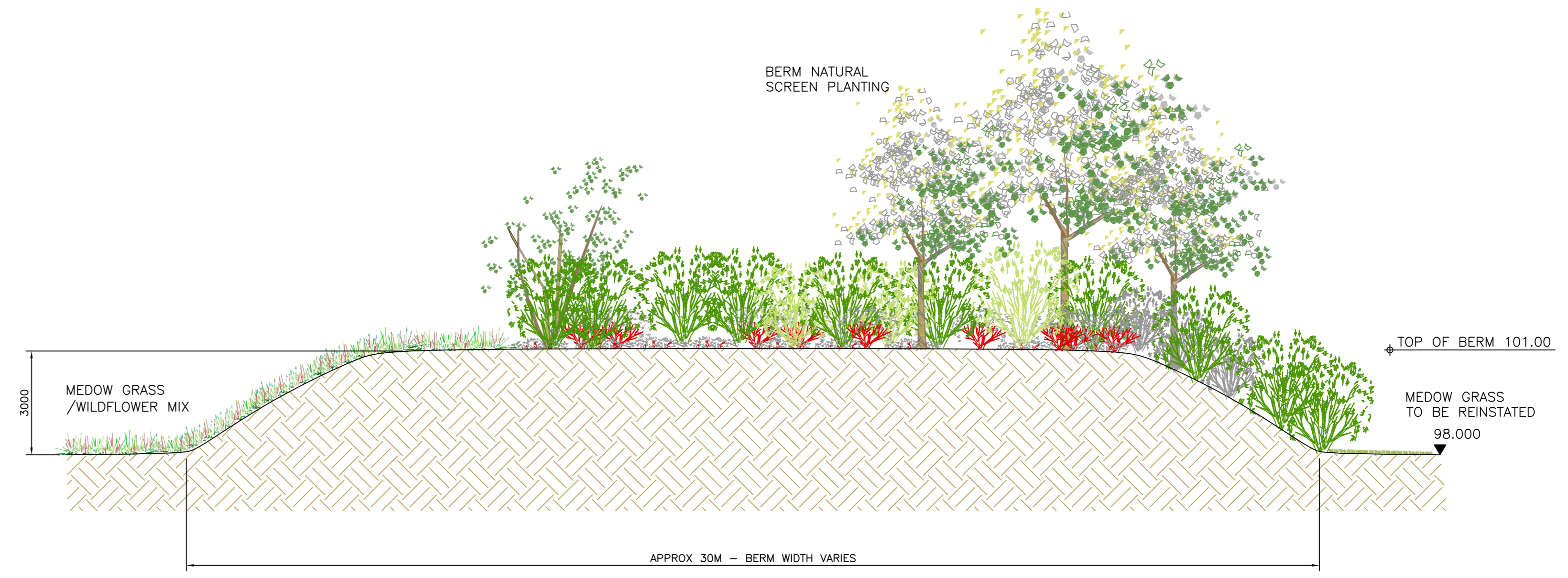
TYPICAL PLANTING SECTION THROUGH BERM 1:100
